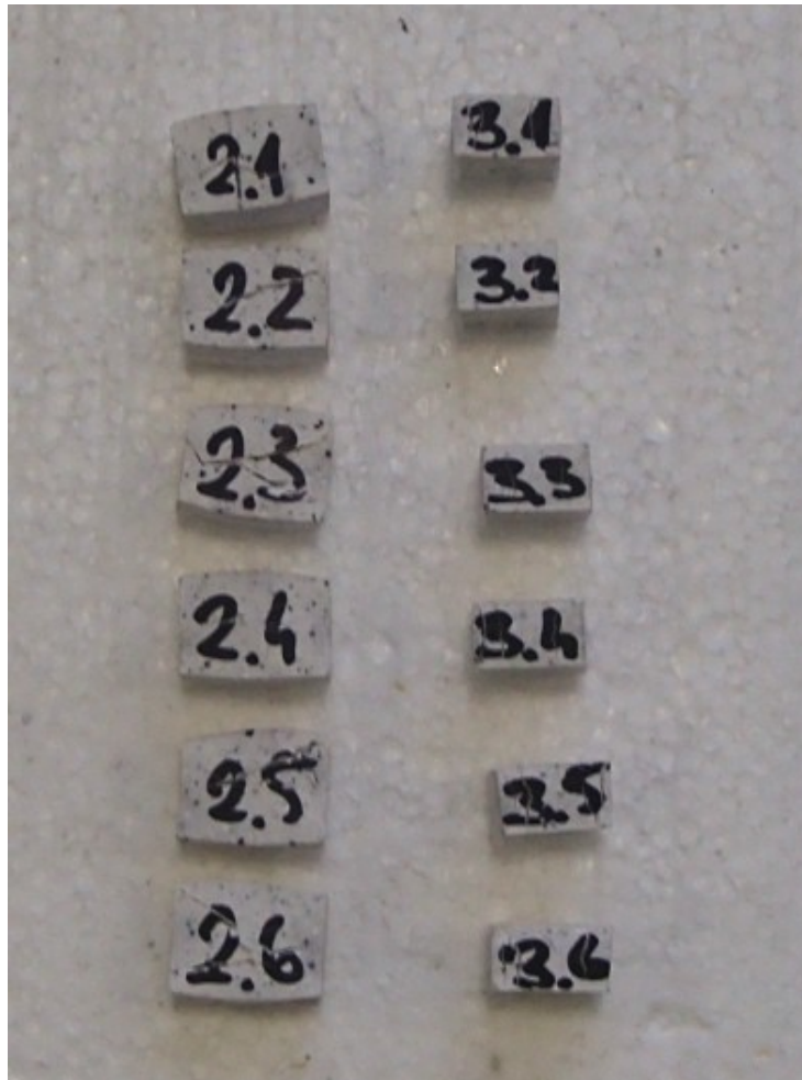
Figure 7. Compression specimens after testing.
