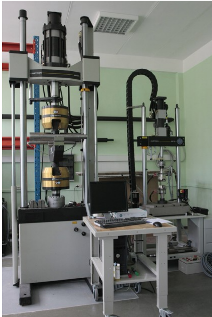
INSTRON 8002 servo-hydraulic test system
