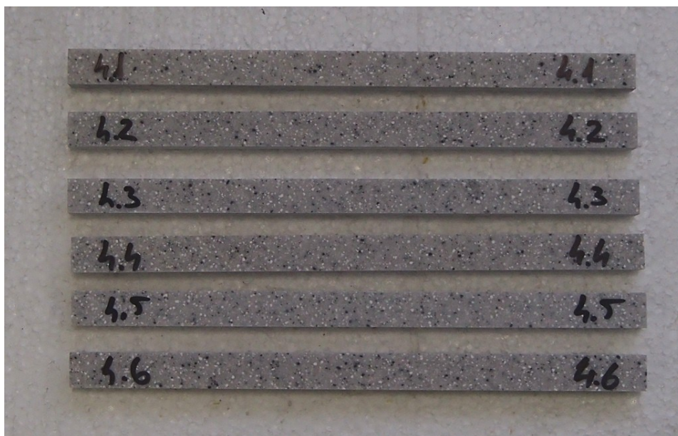
Figure 10. Test specimens for flexure tests.
